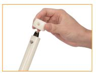
5. Remove the kit from the Connecting rod shaft ⑥
