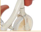
11. Hook one end of the fixed shaft into the reserved hole on the front wheel 2
