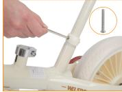
8. Tighten the short screw to secure
