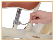
9. Install the bicycle seat<sup>5</sup>. Adjust it to the desired height, then tighten the locking screw securely
