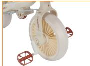
18. The pedal (9) can also be installed on the front wheel (2)
